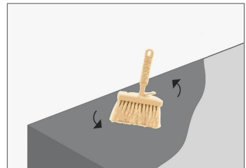
**NOTE:** For a smoother, stucco like finish, allow the applied product to set for 5-10 minutes, then smooth the surface with one or two light passes with a trowel.
