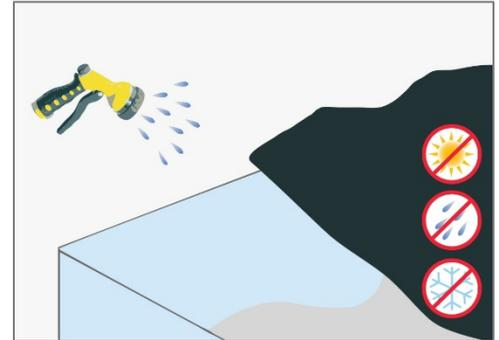
**IMPORTANT:** Freshly applied Krystol T1 must be protected from early drying, rain, frost and traffic. Once hardened it must be kept damp and wet cured for at least 3 days to develop its full properties. Longer curing periods are beneficial.
